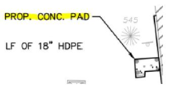
Answer: Concrete pad shall be 6" Concrete. Please refer to 'Standard Duty Concrete' detail on sheet C301.
