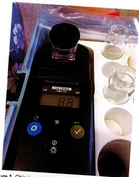
Picture 1. Chlorine residual from women's bathroom was higher than the upper detection limit for the instrument used (8.8 ppm).
