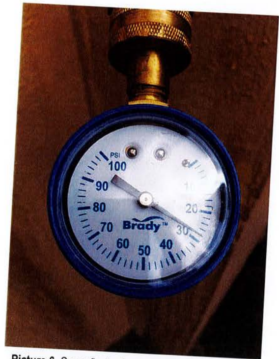
Picture 6. Some fluctuation was observed during the course of the pressure reading. Pressure reading taken from hose bibb on south corner of main building showed a lower gauge pressure of 28 psi.
