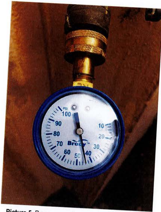
Picture 5. Pressure reading taken from hose bibb on south corner of main building showed an upper gauge pressure of 44 psi.
