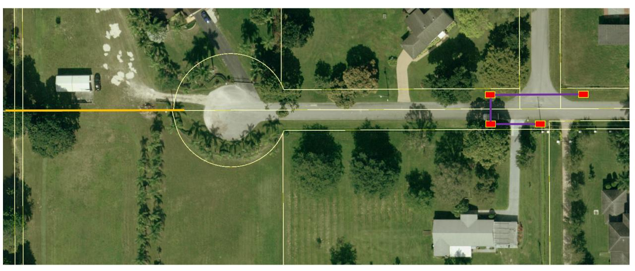
Proposed InletProposed PipeExisting Pipe
