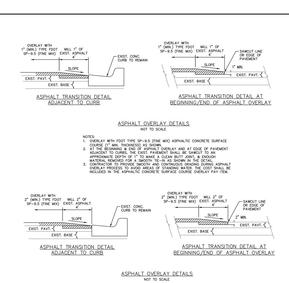
1. OVERLAY WITH FDOT TYPE SP-9.5 (FINE MIX) ASPHALTIC CONCRETE SURFACE
