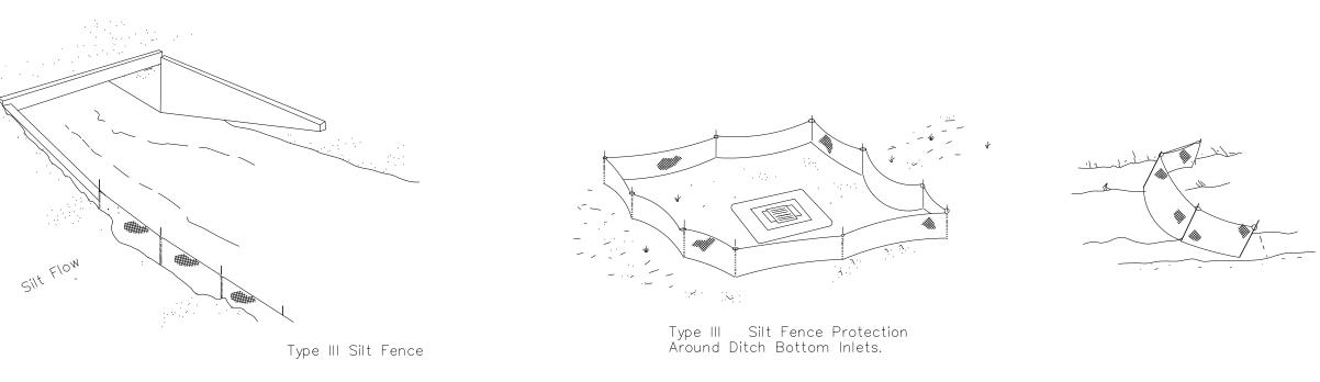
Do not deploy in a manner that silt fences will act as a dam across permanent flowing watercourses. Silt fences are to be used at upland locations and turbidity barriers used at permanent bodies of water.
